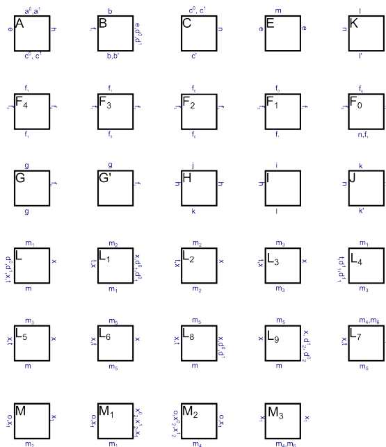
Figure 4.11: The tile types that are used in the construction of a thin rectangle and their respective glues (signals are not shown in this figure). The tile types in the top three rows are used in Step 1, and the tile types in the bottom three rows are used in Step 3. The power of all the glues is \tau/2 , where \tau is the temperature of the DTAM system, except for the glues t , k , k' , l and l' whose power is \tau/3 . (Note that glue superscripts 0 and 1 are only used in this figure, to simplify the explanation for the glue strengths. That is, the presence of d^0 and d^1 on the same edge only indicates that glue d is present, and that its strength is the sum the individual strengths of its components d^0 and d^1 , both of which have strength \tau/2 ). Functionally, glues x , o , t , d , d_2 , d_1 are used for the attachment of columns, while glue m with different subscripts is used for the attachment of rows. Glue f with different subscripts is used for the attachment of the counter. Table 4.1 and Table 4.2 include the detailed definition of the signals and transitions for all these tile types.
